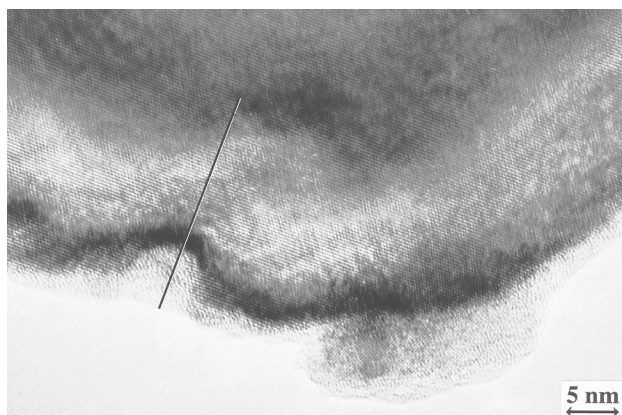
Fig. 5 HREM image of a single BaTiO 3 particle partially exhibiting an amorphous surface layer of ca. 3–5 nm in thickness
